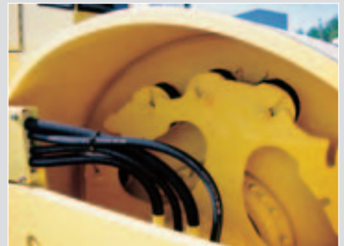
Individually changeable rubber buffers with no special tools or disassembly of the drum required
